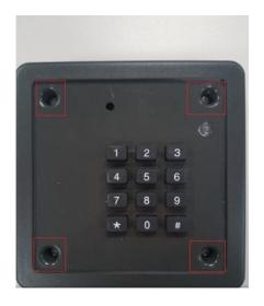
2. Remove the four screws securing the cover.
