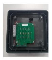
4. The keypad is split into two parts which are the rubber keypad portion and the PCB / CCA that is connected to it. The back of the rubber keys has metal contacts that when pressed will connect with the PCB / CCA that activates a button.
