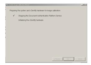
This screen prepares the computer and the *i-D*entify hardware for calibration. The process includes stopping the AssureID Service and then initializing the *i-D*entify hardware.
