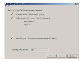
After the wizard has completed calibration, it displays the serial number of the *i-D*entify hardware that has been calibrated. At this point the user may click the **Finish** button to complete the process and exit the calibration wizard. The computer is now ready to run the AssureID applications with the calibrated *i-D*entify hardware.
