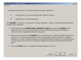
When the wizard has completed preparation, the user is instructed to insert the calibration target. It is very important that the calibration target is flat on the glass platen and flush against the back and left edges. Follow the directions in the application and then click the **Next>** button to begin calibration.
