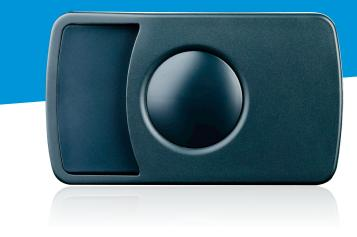
The Prox Booster is a vehicle and driver identification tag. This patented solution ensures that a vehicle can only get access to a secured area when driven by an authorized driver. The Prox Booster is used in combination with (existing) personal access credentials. Based on semi active RFID technology, the Prox Booster is identified up to 12 meters\* (40 feet) with the TRANSIT Ultimate reader.
